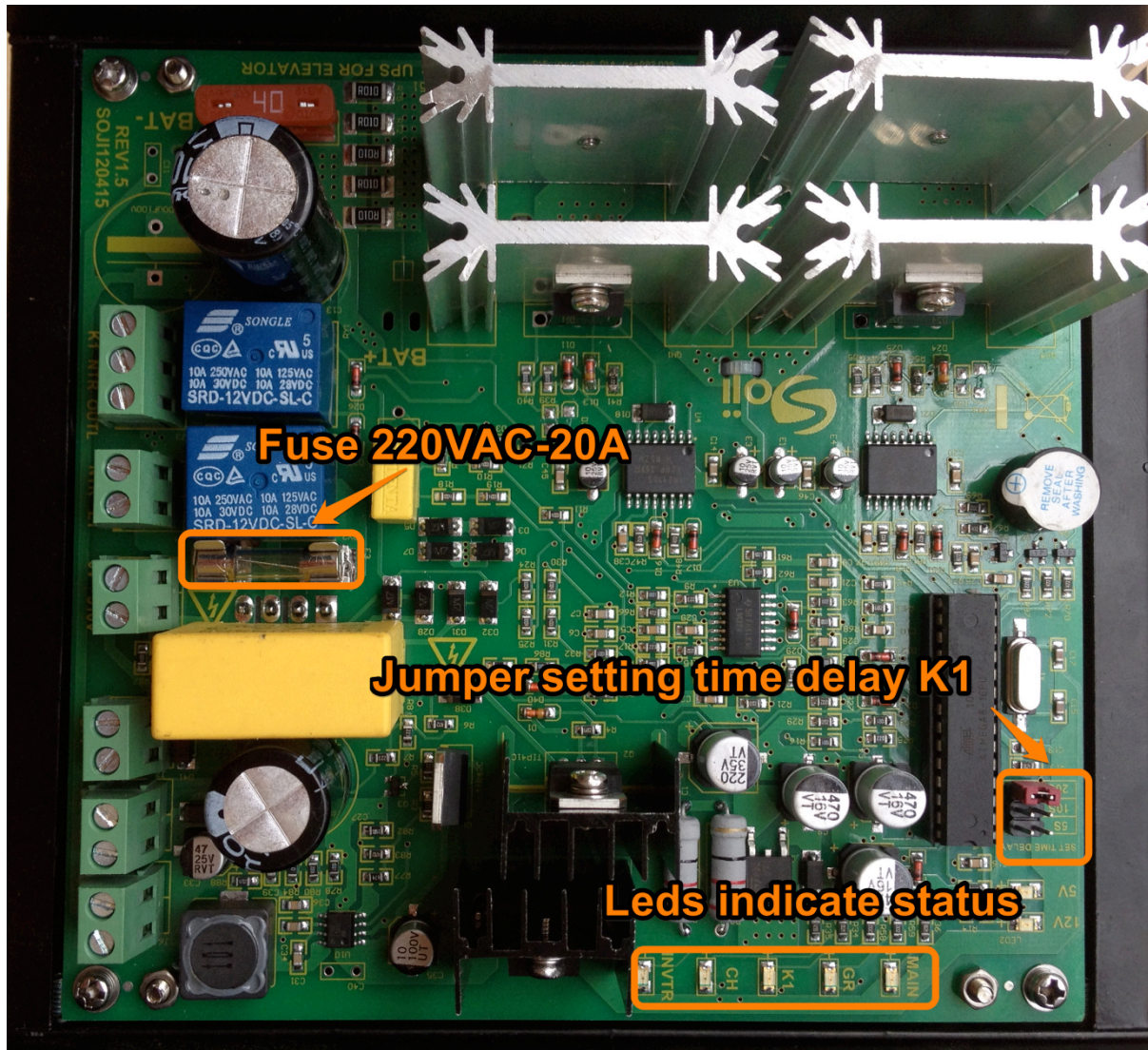
Main PCB of Elevator rescue device SOJI SP Series
